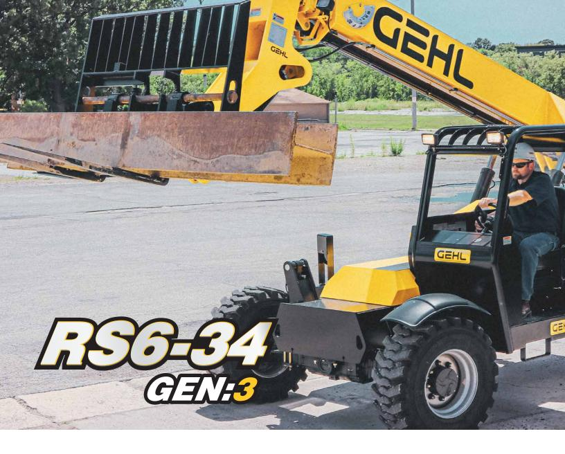
The RS6-34 GEN:3 has a unique reach to its RS brothers and sisters in the lineup. With a 34' maximum lift and 6,000lb lift capacity, this Telescopic Handler is ready to serve you and its response time will outshine any coworker you have. Push the power to its maximum effort and get the job done the way you need, because this machine Works Like You.
