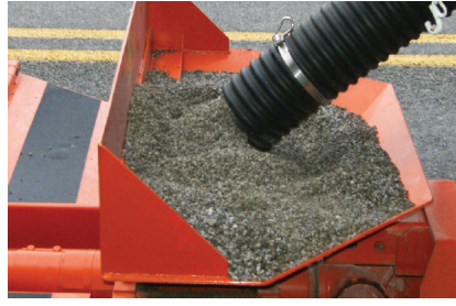
Gravity feed aggregate delivery
