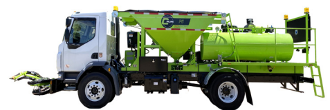
P5 One-Person Patcher with DuraPatcher™ Technology
