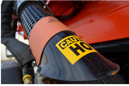
Vent-Flo™ nozzle with optional heater
