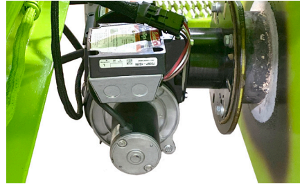
340,000 BTU Diesel Material Tank Burner
